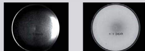
Object: Bottom of aerosol can. Uniform illumination of concave surface results in contrast against printed characters.
