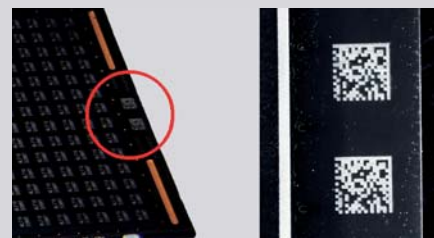
Object: Circuit board. Image captured shows high contrast Data Matrix symbols.
