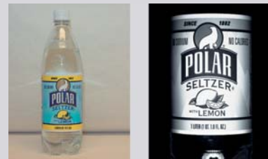
Object: Labeled bottle. Inspect for label presence or absence, correct label and proper orientation.
