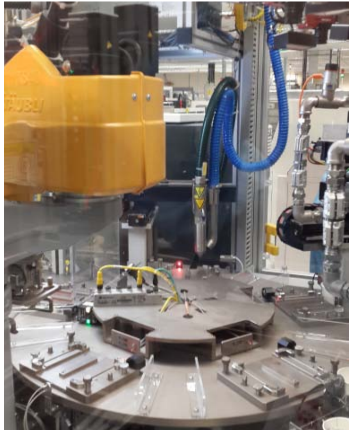
Microscan's Vision HAWK is integrated into a robot arm for vision inspection on the assembly line.
