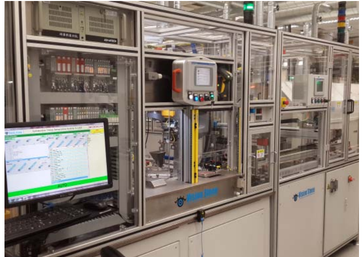
Vision Stone developed and installed a custom-made vision inspection system for TRW with multiple smart cameras from Microscan.
