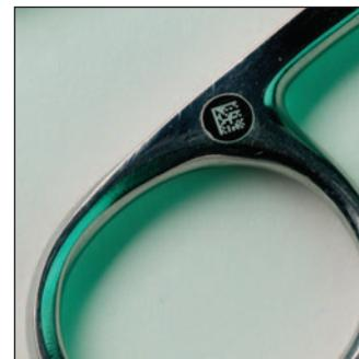
This direct part mark example shows a laser etch 2D symbol (Data Matrix) on a metal medical device.
