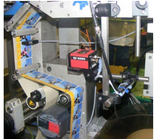
A barcode system can be used to validate labels prior to final packaging.
