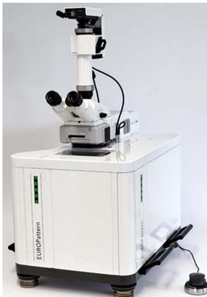
Microscan's MS-4 imager is integrated inside the EUROPattern Microscope.
