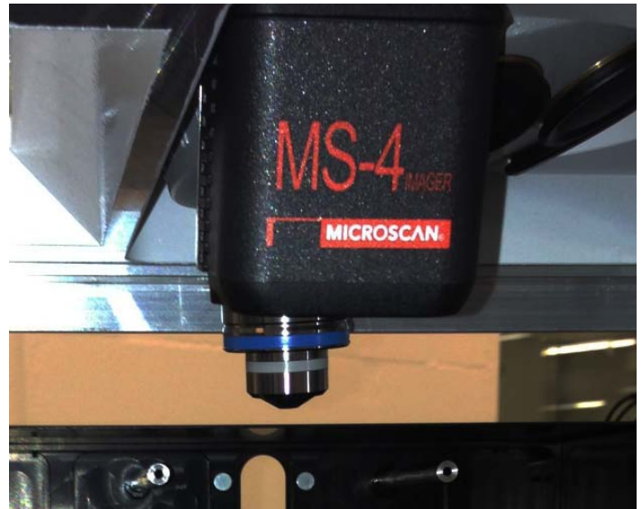
The MS-4 imager decodes the Data Matrix code on the microscope slide inside the EUROPattern Microscope.
