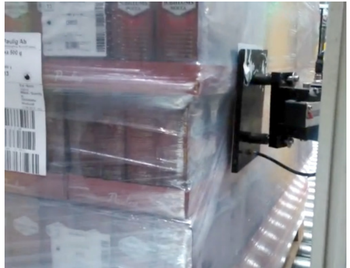
Microscan's QX-870 Raster Laser Scanner validates the barcode on the pallet label immediately after it is printed.
