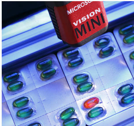
Figure 6: A machine vision camera inspects blister packaging for accurate pill presence and color.
