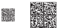
Figure 13: How close does the device need to be to read this 5 mil code and 10 mil code accurately? The key is having the appropriate optical envelope.
