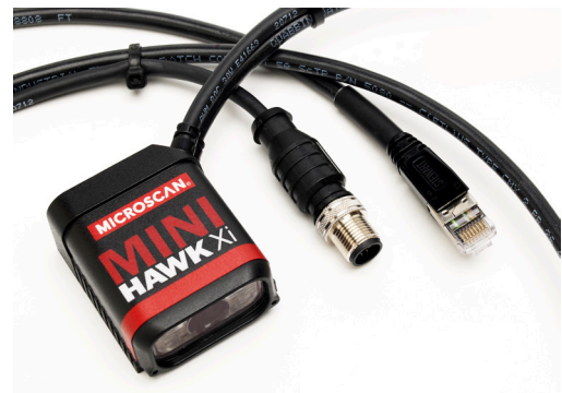
Figure 14: Devices that offer multiple connectivity options, such as RS-232 and Ethernet (shown above), provide additional flexibility in embedding.
