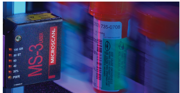
Figure 8: A laser scanner integrated into a clinical sample tracking and traceability system achieves up to 1,000 decodes per second.
