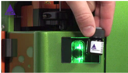
Figure 9: A barcode imager embedded within a clinical analyzer logs samples presented by a human operator.
