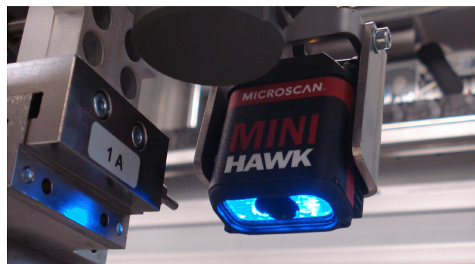
Figure 1: A compact barcode imager embedded into PCB labeling and printing machine logs product data and ensures barcode presence.
