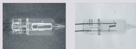
Object: Light bulb. Resulting image clearly shows silhouette of filament inside the bulb.
