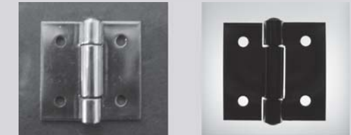
Object: Metal hinge. Backlighting allows high contrast image of drilled holes.
