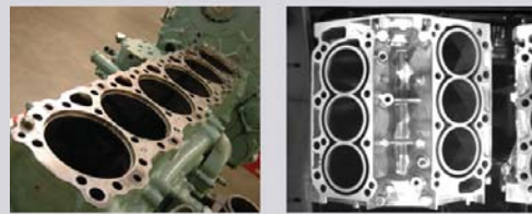
Object: Large engine block. Provides good contrast over large areas to perform product inspection.
