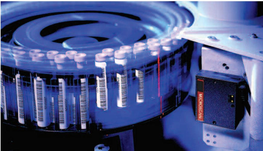
Figure 10. Through a combination of solid-state technology and LED-based illumination, megapixel imagers extend the life expectancy of the bar code reader subsystem.
