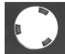
Reflection from Ambient Light Results in Inaccurate Cap Measurement
