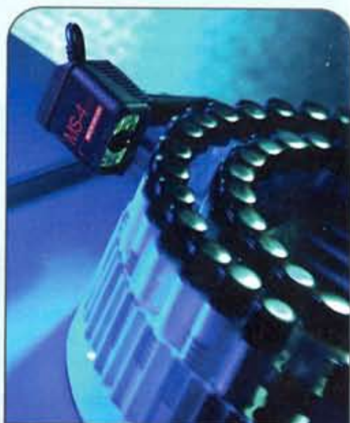
A solid-state imager can accurately decode both linear bar codes and 2-D symbols.
