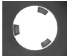
Infrared Light Removes Unwanted Reflection
