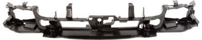
**A typical grille opening reinforcement.**
