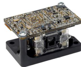
**The MS-2D engine provides the best performance available for reading 1D/2D symbols and direct part marks at very close range.**
