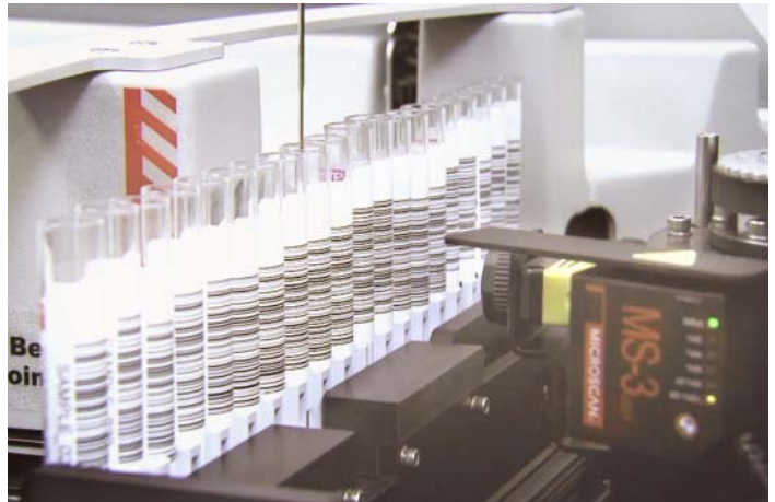
Strategically placed MS-3 Laser Scanner identifies specimen samples.
