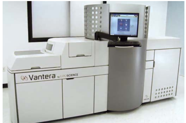
The Vantera Clinical Analyzer performs sophisticated NMR-based lipoprotein analysis and uses Microscan's MS-3 Laser Scanner to identify and track samples and diluents.
