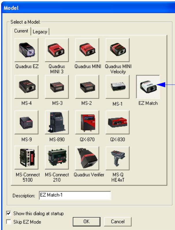
**Important:** An EZ Match Imager must be connected to the host computer for its corresponding icon (shown at left) to appear on the model menu.
