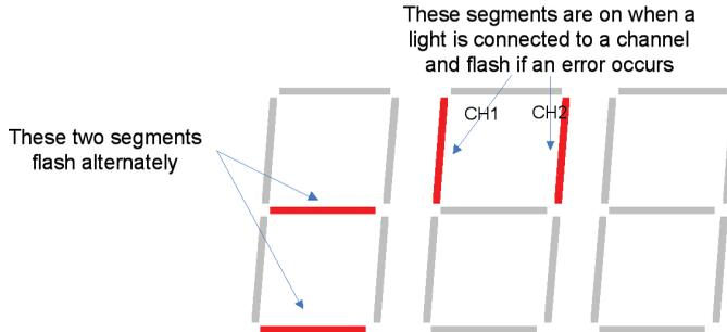
Errors are usually caused by a light being connected but the rating for that light has not been set. The rating of a light can be set as described in Section 7.1.
