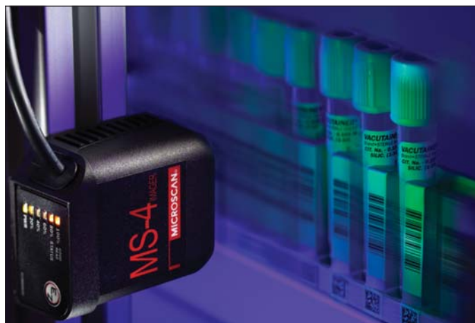
Figure 1. Miniature megapixel imagers quickly read multiple 1D and 2D codes in a single image capture for highly efficient data acquisition.
