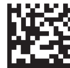
Figure 3: This 2D Data Matrix ECC 200 symbology is infinitely scalable.
