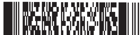
Figure 2: PDF417, an example of a stacked symbology, is composed of stacked rows of width modulated barcodes.
