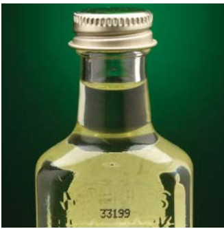
OCR can be used to confirm that every product is marked with the appropriate text string before exiting the factory.
