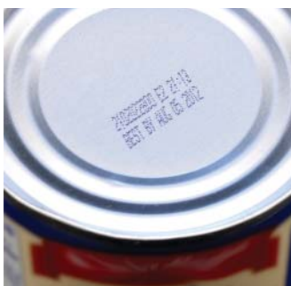
OCR characters printed on the top of cans are used to make sure that the correct label is put on the can.
