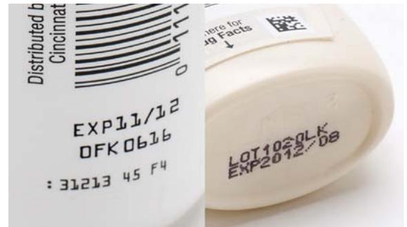
A crisp OCR font (left) is the simplest and most reliable method for decoding, while more challenging marks such as the inkjet mark on the bottom of the bottle (right) can be read using teachable OCR systems.
